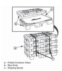
Step 3: As needed, stack as many as sixteen cradles together. Place three or more stacks inside an empty *un-collapsed* container. Band for shipment.
