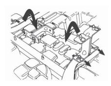
Step 2: Position folded sides of container on base. Place top cover over base assembly. Stack *no more than four* complete assemblies together and band for shipping.
