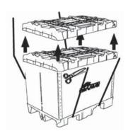
Step 2: Remove the four metal corner posts and place in underside of top cover.
