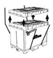
Step 2: Remove the four metal corner posts and place in underside of top cover.
